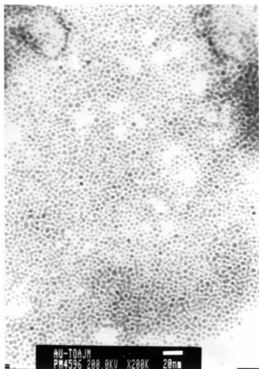
Figure 2. TEM image of TA-derivatized gold nanoparticles after transfer into water.
